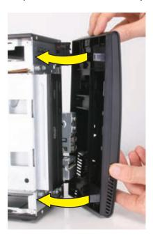
**10** Align the tabs on the inside edge of the left side panel with the slots in the edge of the left side of the computer case.
